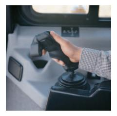
**Work Tool Controls.** The D6R II features ergonomically designed blade and ripper controls with low effort pilot operated hydraulics for added operator comfort, easy operation and precise work tool control. When equipped with a PAT blade, the blade control allows simultaneous six way control of the blade with a thumb rocker control to adjust blade angle.
