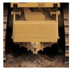
**Rear Counterweight.** Rear counterweights may be needed to optimize balance for backing up steep slopes or increasing performance in heavy dozing applications. Recommended if other rear attachment is not specified.
