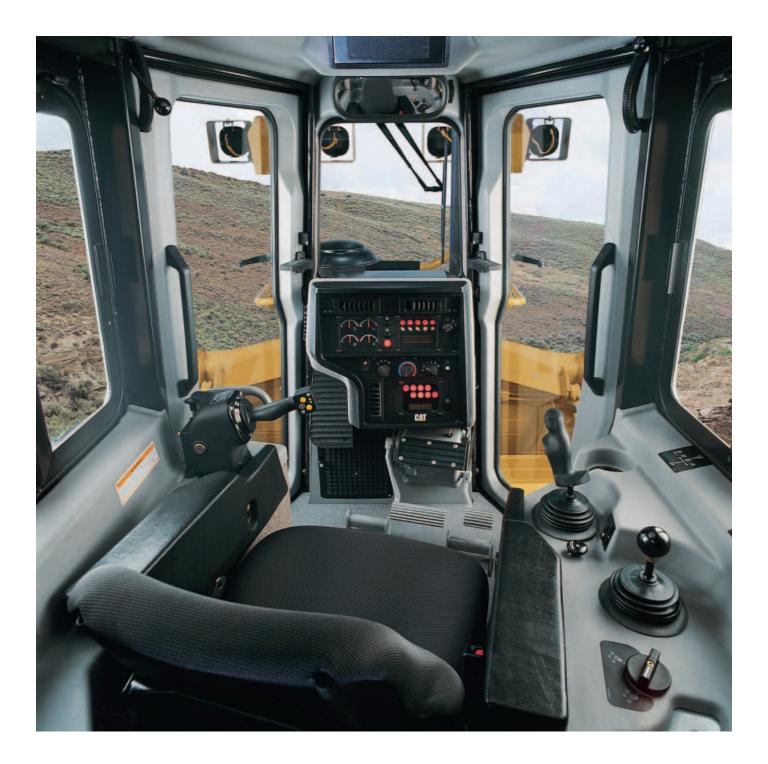
**Cab.** Isolation-mounted, pressurized cab reduces noise and vibration for operator comfort.
