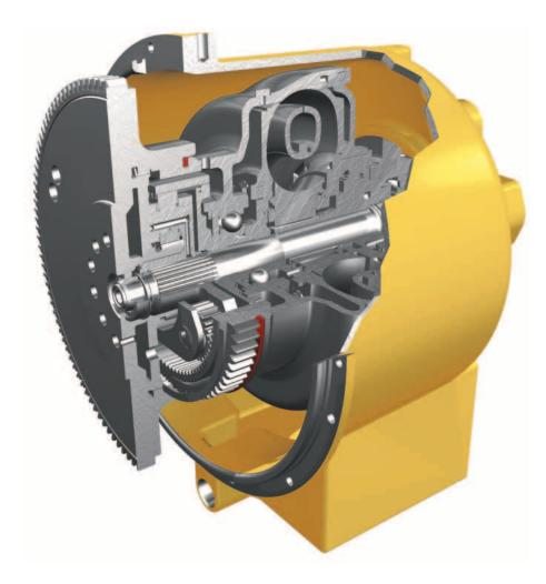
**Torque Divider.** A single stage torque converter sends 70% of engine torque through a converter and 30% through a direct drive shaft for greater driveline efficiency and higher torque multiplication to get heavy loads moving. The torque divider provides improved efficiency and broader range of performance in second gear applications.
