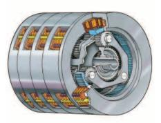
**Transmission.** The D6R II planetary power shift transmission features three speeds forward and three speeds reverse and utilizes large diameter, high-capacity, oil-cooled clutches. To maximize the life of the transmission, the planetary design distributes loads and stresses over multiple gears.
